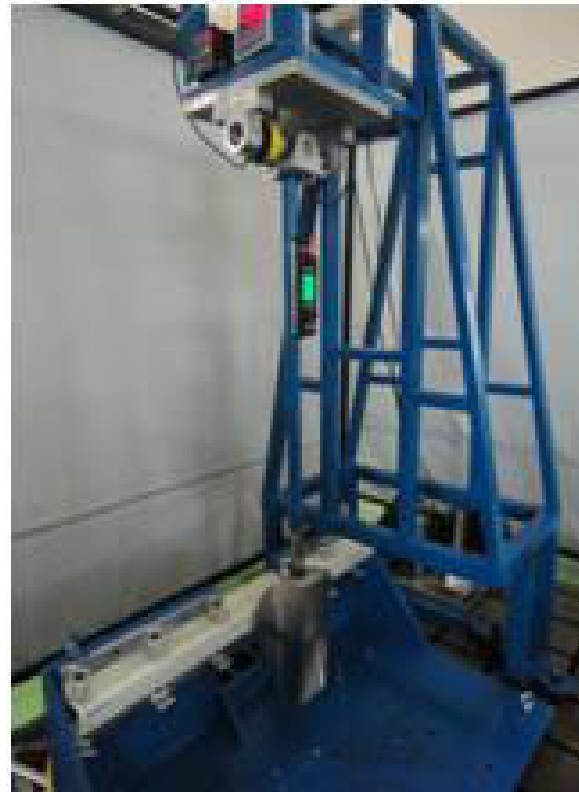
Fig. 5. Impact loading bending test machine
